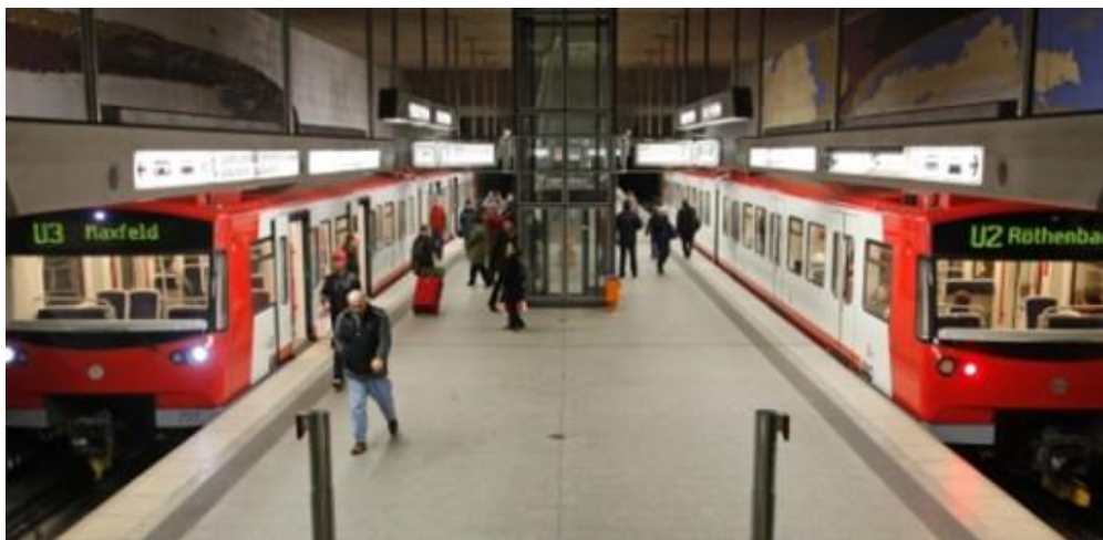
Fig 6: Automatic metro trains in Nuremberg without platform screens. This has allowed the transport authority to run driver operated trains in the same tunnel.
