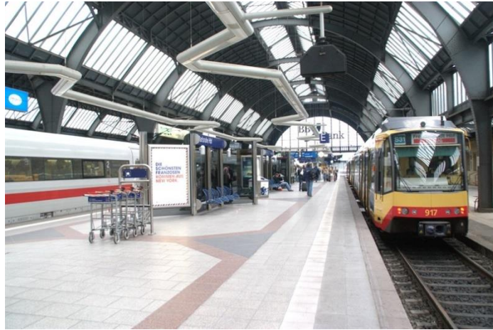
Fig 26: To the right there is a tram train which can also use heavy rail track on the same platform of an Intercity train. Note the moveable steps to bridge the gap to the platforms.
